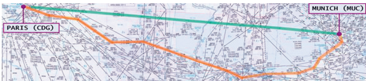
On this route above, an airplane would fly 680 km on the green direct path. Actually, the distance flown (orange path) is 910 km.
